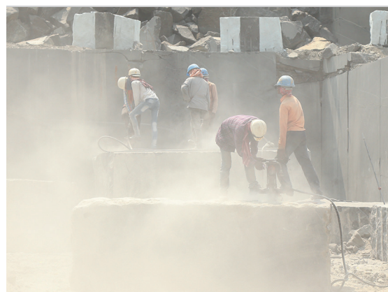
Respiratory disease, such as silicosis, can be a cause of illness and death in some sectors.
