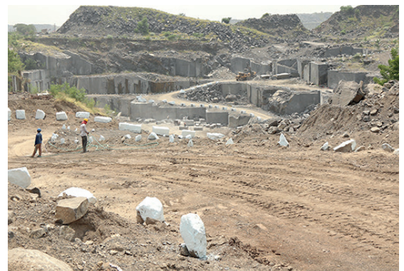
Silica dust on floor of quarries can become airborne in the wind - water should be sprayed on the ground to prevent the dust from rising
