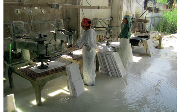
These workers are in a ventilated area, and are using water. However, should also be using dust masks
